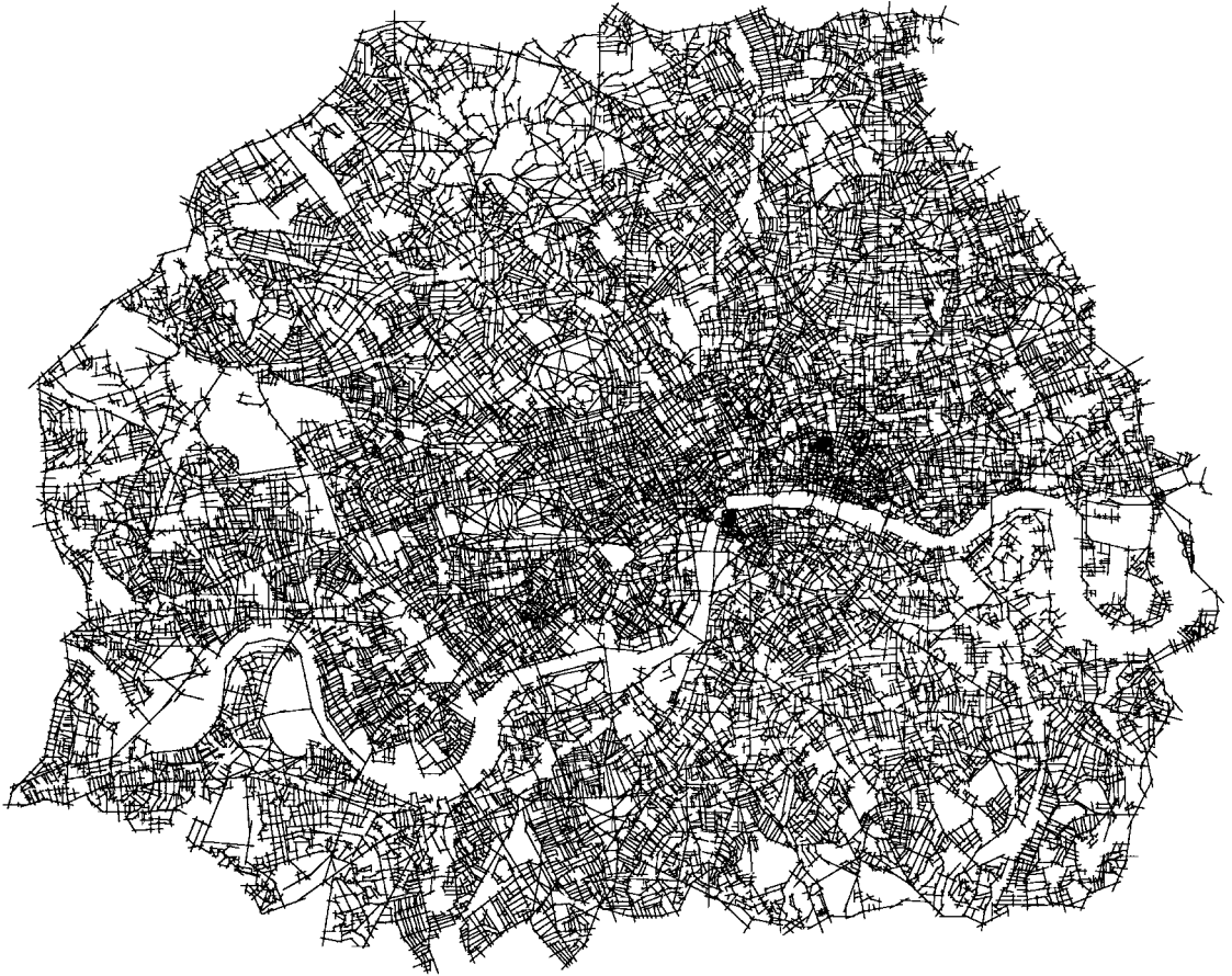
FIGURE 28.5 Axial map of Greater London within the North and South Circular Roads.
